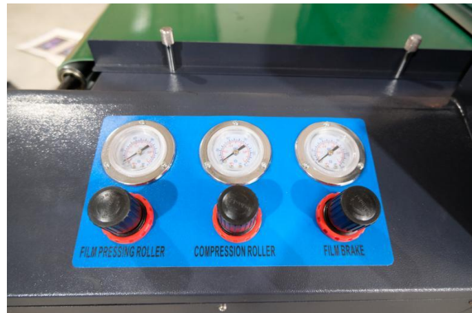
AIR PRESSURE CONTROL PANEL
